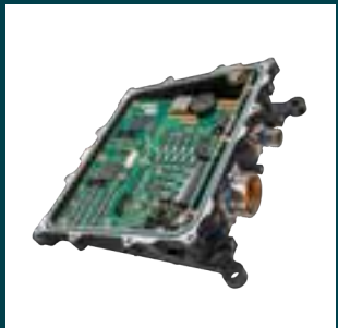
AVIONICS COMPUTER High-performance computer for highly automated regulation and control tasks like autopilot.
